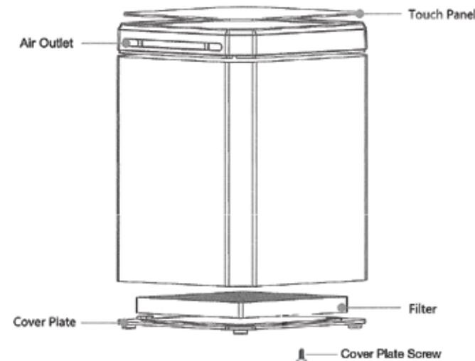
NOTE: Tighten screws on cover plate after replacing filter.
