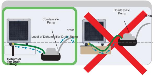
IMPORTANT: The drain hose from dehumidifier to pump must run downward and stay below the level of dehumidifier drain fitting.
