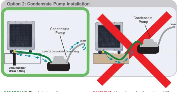
**IMPORTANT:** The drain hose from dehumidifier to pump must run downward and stay below the level of dehumidifier drain fitting. Tubing line from pump can run up to 20 feet upward and out into drain.
