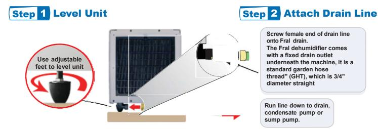
Note well: If the machine does not have adjustable feet, check that it is properly leveled.
