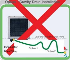
WARNING: Double siphon is not allowed because it not allow correct drainage of water
